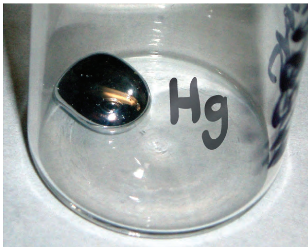
Figure 2.13 The symbol Hg represents the element mercury regardless of the amount; it could represent one atom of mercury or a large amount of mercury.
