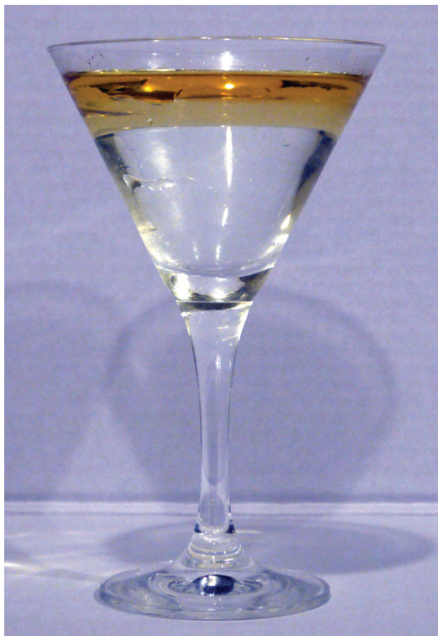
Figure 11.15 Water and oil are immiscible. Mixtures of these two substances will form two separate layers with the less dense oil floating on top of the water. (credit: “Yortw”/Flickr)
